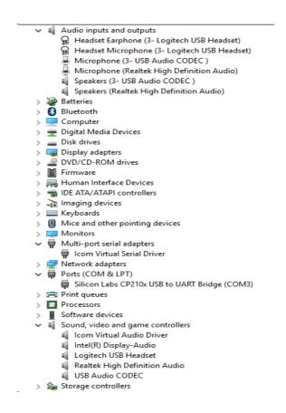
**A. Windows Device manager** – This is a screenshot after installing the USB driver package from ICOM, which supports the US audio and serial comms hardware built inside the IC-7300. Audio inputs & outputs (USB Audio CODEC), Multi-port serial adapter and Ports (COM & LPT) should show the following entries if you have installed the ICOM USB drivers correctly (i.e. before connecting the USB cable – see "additional Notes").
