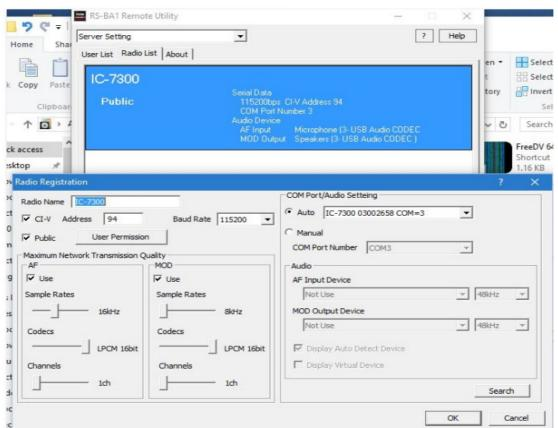
The radio name is what the remote control program on the REMOTE PC will see when LOCAL and REMOTE PCs are connected. Set all other settings as shown. If the auto Com port setting does not reflect the port from the Windows device manager, it can be set manually.
