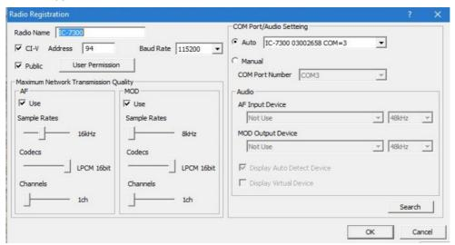
D. **Remote Control program -** *connection settings* – connection type USB and speed 115200, C-IV address 94 and the com port is the one displayed in the Windows device manager under the Silicon Labs CP210x entry.
