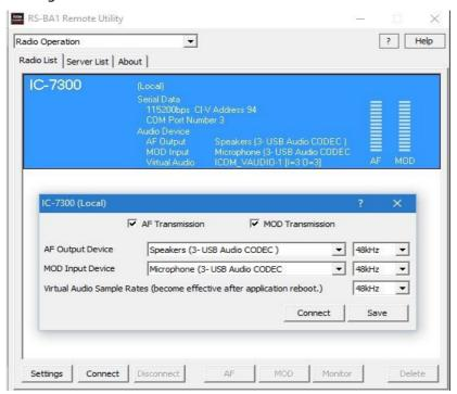
**E. Remote Utility program on LOCAL PC -** Radio operation / Radio list. Operational view - this shows who is connected remotely. NOTE: you should NOT connect using this program on the IC-7300 from the LOCAL PC, doing so will block the remote station! In the example shown ASUSEEEPC900HA is the REMOTE PC.
