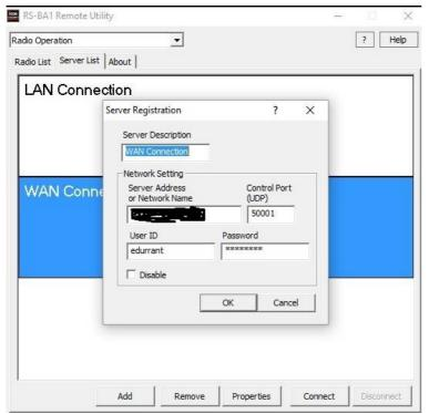
The blacked out field will contain either your Internet static IP address if you have one or the domain name of your domain defined on a Dynamic DNS service provider such as DYNDNS or NOIP. The control port will need to change only if you have had to change the ports in use in
