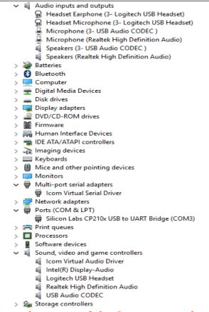
→ make a note of the Com port number on the Silicon Labs CP210x line ←
