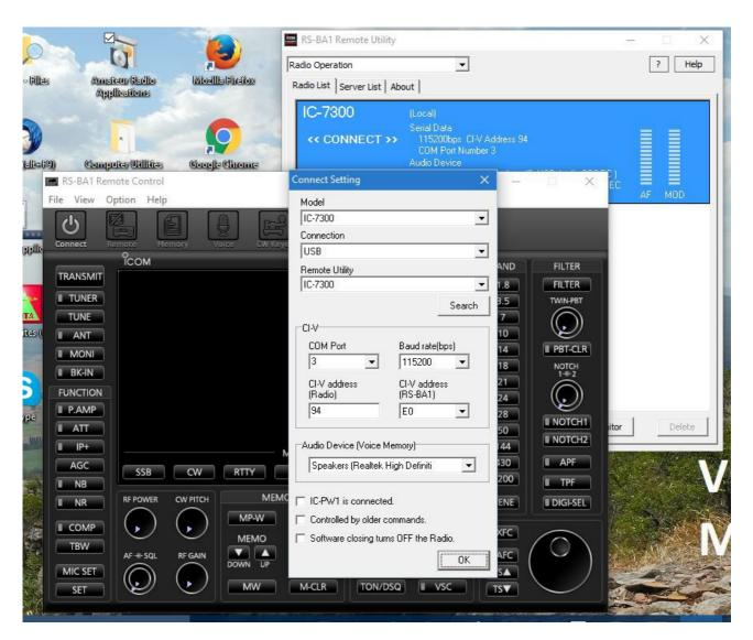
4. Once saved close both the remote control program and the remote utility and then follow the standard start process - for a "Non-remote" - control from the shack process, this is to start the remote utility, press connect and if all is OK, then go to the Remote control program, start that and press connect there.
